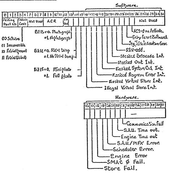
The parameter for interrupts other than on the current OCP port will look like an empty software failure parameter (i.e. bits 16-31 not used).
