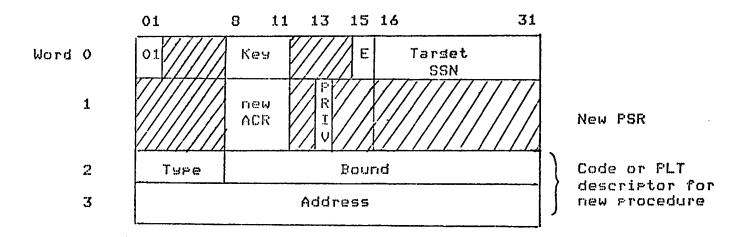
The Key is checked against the caller's ACR. If satisfactory, the procedure defined by the descriptor is entered on the new stack with B, C and the parameters set up on the old stack. A special inward return scriptor is set in the LINK field of the new stack which does the converse. ACC and B are preserved across an inward return so that it is possible to outward call Function and Maps if desired.
