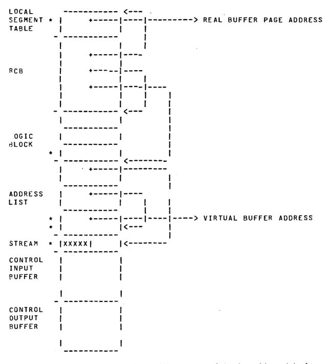
NOTE: Words marked with a \* need to be altered before each stream transfer. All other words can be settup on adaptor initialization.
