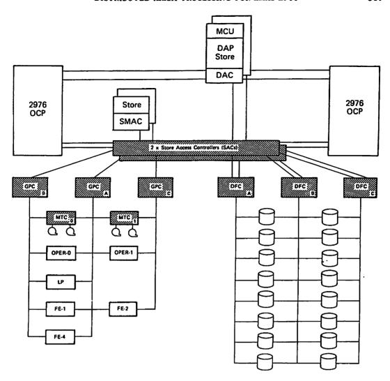
Key: OCP - Order Code Processor GPC - General Peripheral Controller DAP - Distributed Array Processor MTC - Magnetic Tape Controller DAC - DAP Access Controller **OPER - Operator Console** MCU - Master Control Unit LP - Line Printer SAC - Store Access Controller FE - Front End SMAC - Store Multiple Access Controller (Communications Processor) DFC - Disc File Controller Mbyte - 1,048,576 bytes
