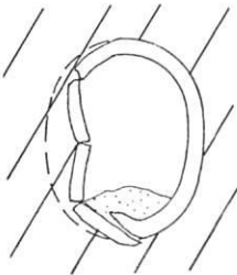
3) Side wall fails in bending
