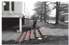
Obstacle: Main steps joining upper and lower concourses, ramp to side unsuitable for wheelchair users due to steep gradient.
