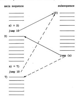
In the same way the instruction n) = m) makes a jump (n) instruction transfer control to one of several different points depending on the computed value of m. This device is known as a multi-way switch. When an index is used to 'remember' a label in this way it cannot, at the same time, be used for other purposes.
