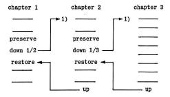
A consequence of this arrangement is that any results calculated by the subchapter will have to be recorded in the auxiliary store in order to preserve them. Alternatively, if they are left in the working store, then the *restore* instruction can be postponed until they have been dealt with in the master chapter.
