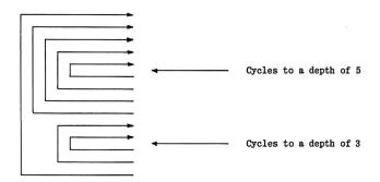
This example is typical and illustrates the type of flow arrangement which is permissible. Note that no lines cross.
