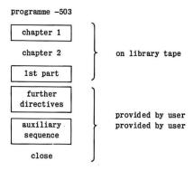
In such a programme it is obviously necessary to know how much of the chapter space is available for the auxiliary sequence, what labels can be used, and so on. It is convenient to assume that it would be entered at the first instruction and terminated by returning control to a preassigned point in the first part of the chapter, e.g., label 127.
